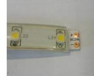
Silicone-free connecting-/soldered joint of the flexible LED tape.
