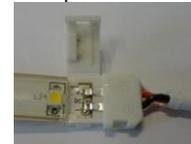
Easy, silicone-free connector: slide connecting joint of the Flexible LED carefully under the contact of the connector. Then close strain relief.
