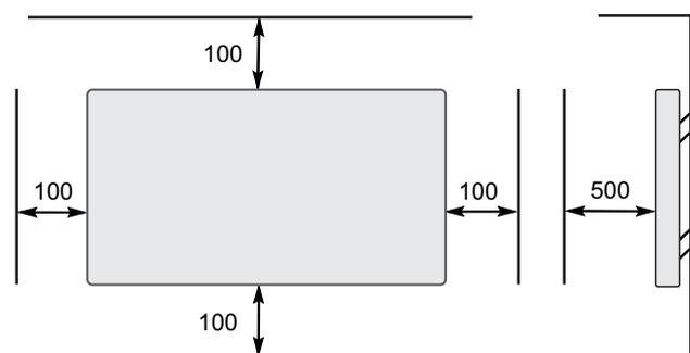
When installing the heating device with mains power socket and room thermostat, the protection zone in accordance with VDE 100-701 must be observed.
