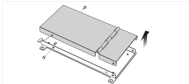
1 Remove screws. Lift cover off.
