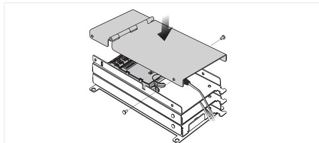
6 To add additional modules, repeat steps 4 and 5. If this is the final module, affix cover of EDGE-SMH-SPLC using two screws.
