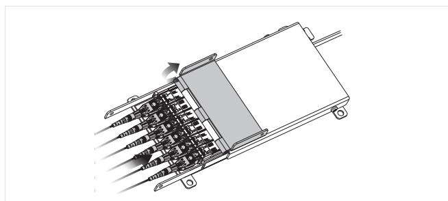
7 Open hinged lid. Clean and insert connectors into cleaned adapters.
