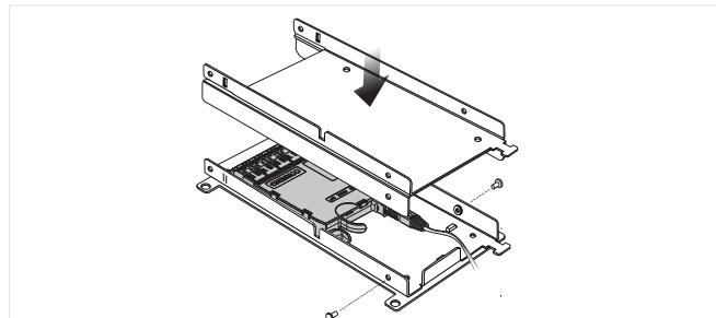
4 Use two screws to attach the EDGE-SMH-XPDR to the EDGE-SMH-SPLC Base.
