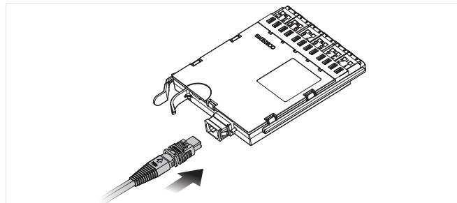
2 Clean and insert MTP connector into module.
