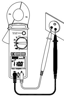
Set the switch to V~ for an AC voltage measurement and to V= for a DC voltage measurement.
