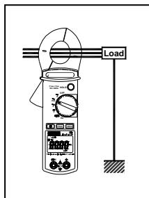
**Note:** As a safety measure, disconnect the measuring cords from the clamp before performing this operation. The measurement is optimal with the conductor centred in the middle of the jaws.
