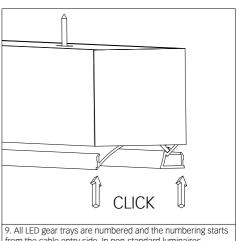
9. All LED gear trays are numbered and the numbering starts from the cable entry side. In non-standard luminaires the numbering of LED gear trays is made in accordance with technical drawings.
