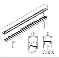
7. All LED gear trays are numbered and the numbering starts from the cable entry side. In non-standard luminaires the numbering of LED gear trays is made in accordance with technical drawings.
