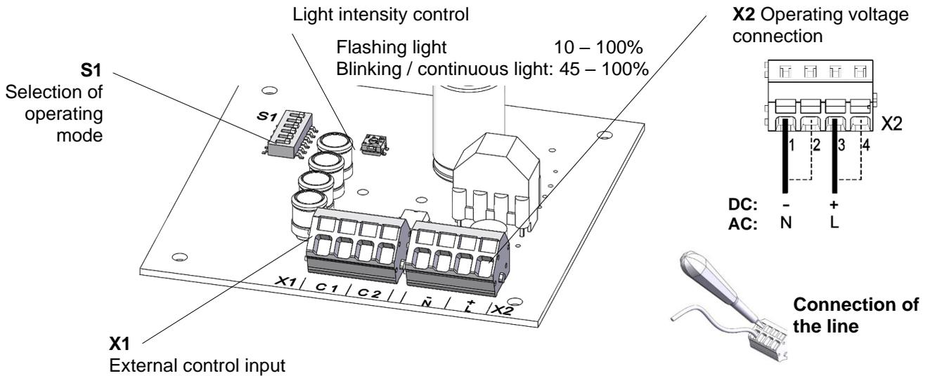
**Note:** Devices with DC voltage are equipped with reverse polarity protection. The function is guaranteed if the polarity of the connections is reversed.
