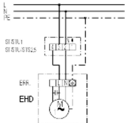
**Radialventilator mit 5-Stufentransformator TRE**
