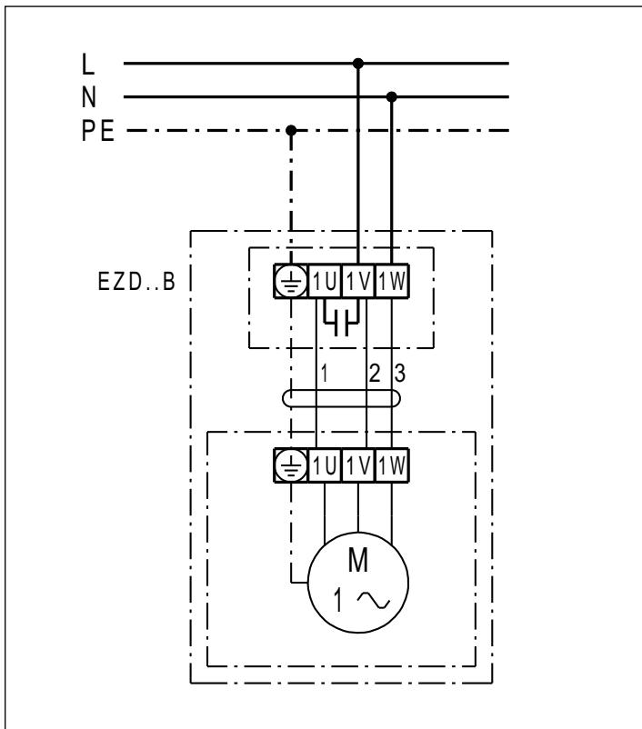
**EZD ... B mit Drehzahlsteller ST../STU../STS..**
