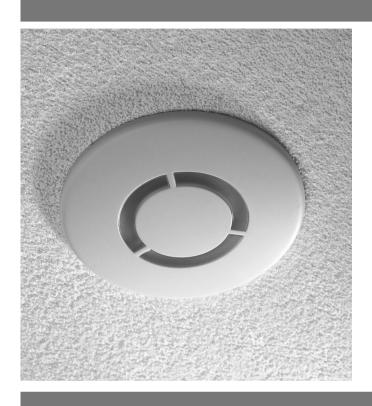
The SWITCHLITE MRE DDM MR microwave presence detector provides automatic control of lighting loads with optional manual control. The SWITCHLITE MRE DDM MR detects movement using a highly sensitive microwave detector. This works by emitting low power microwave signals and measuring the reflections as the signals bounce off moving objects.
