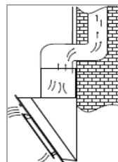
The extracted air is normally vented vertically. The extracted air can be vented through the wall units and the loft floor to the roof ridge.
