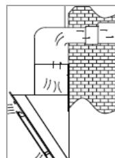
If there is a conduit under the wall units, the extraction duct can be routed so that the extracted air can be vented horizontally through the wall.
