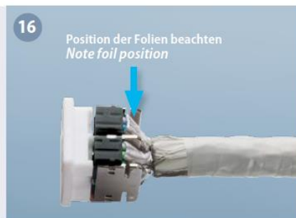
13 Paare in den Wire Manager einführen. Slide the pairs through the wire manager.
