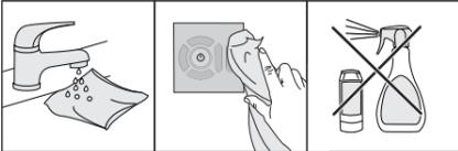
Clean the product with a soft, damp cloth (no microfibers) and utilize only mild detergents and water. Detergents containing chlorine, acid or that are abrasive or corrosive can damage the surface. We cannot accept claims caused by improper cleaning.
